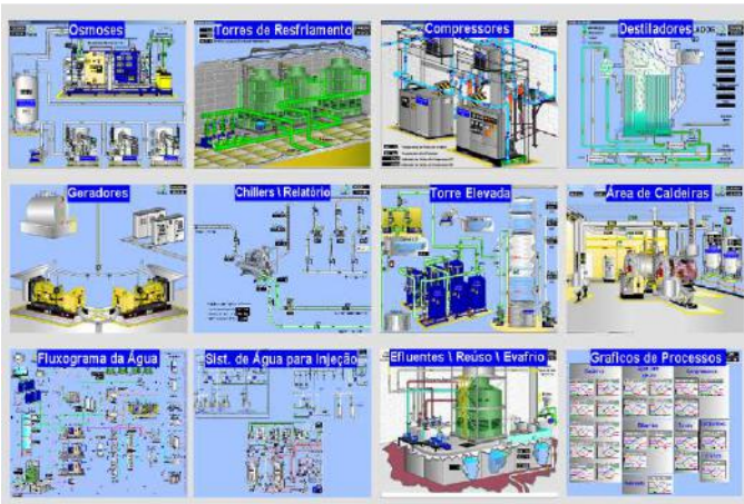
Figure 7. Utilities SCADA System to Monitor Key Process
