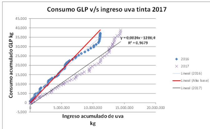
Figure 5: Performance improvements in LPG consumption of the boilers
