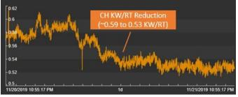
Figure: Lower Inlet Temp. Effect on Chiller Performance
