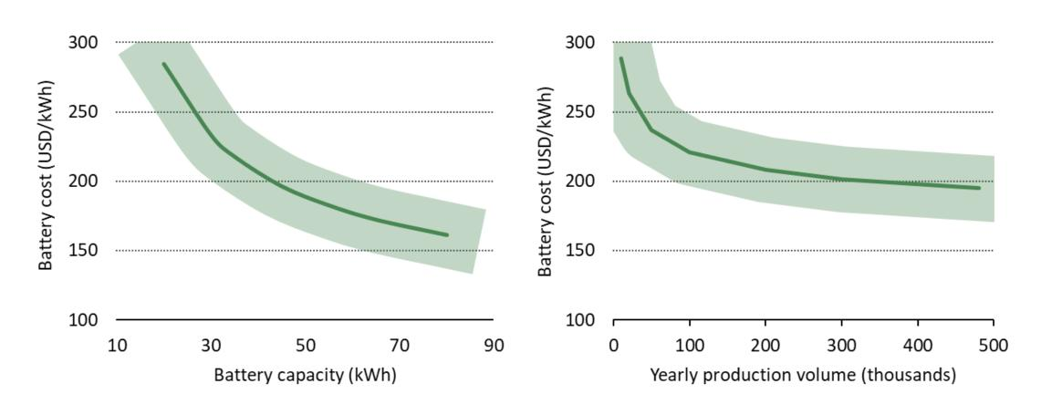
Note: graphics developed for BEV batteries for cars
