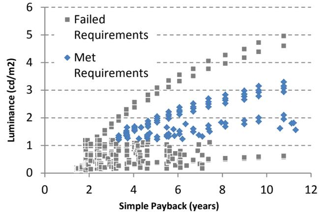
*A Canadian municipality used the tool to identify fixtures that met lighting performance criteria – these were up to 74% more efficient than the existing fixture.*
