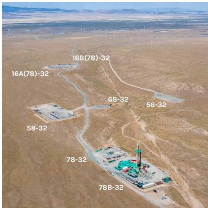
Aerial view of the Utah FORGE field laboratory, showing the layout of production, injection, and monitoring wells across the test site. Source: SLC
