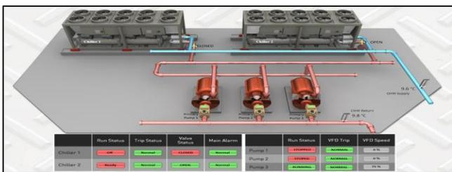
Load based set point reset of the chilled water plant will be varied based on the outside air temperature and load hours such that the water temperature is increased as the cooling requirement for the building decreases. Chiller start / stop will be switched on based on the pull
